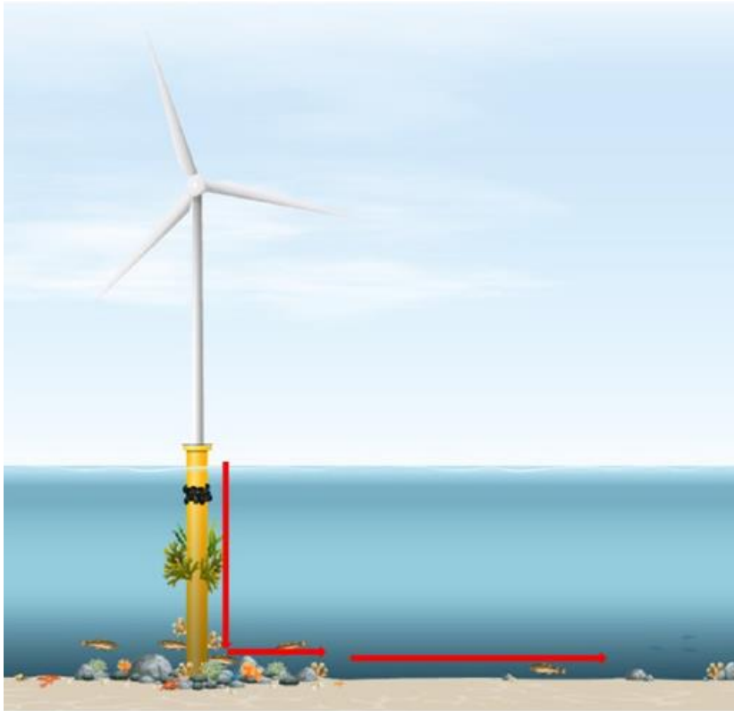
Figure 4. Overview of the wind turbine and ROV survey transects. The figure illustrates the layout of the wind farm, including the scour protection and the transect investigated by the ROV.
