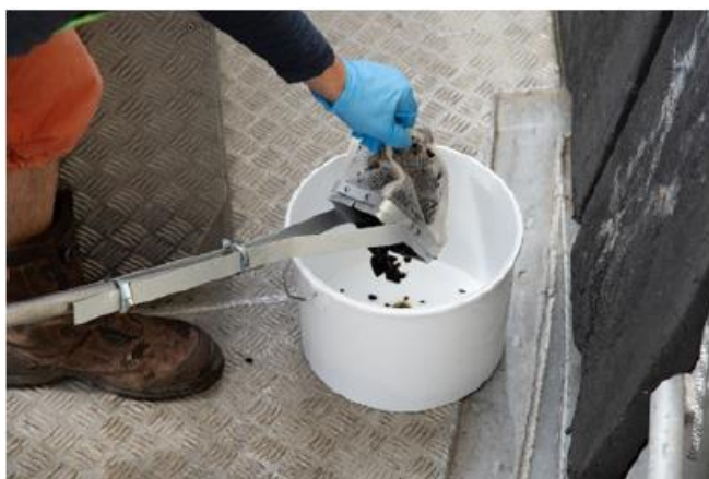
Figure 2. Scraping samples at a turbine tower. Photo: Karsten Dahl.
