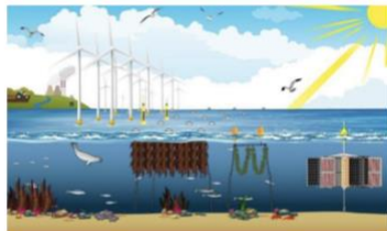
Fig 1 An offshore wind farm (OWF) is a possible multiuse host partner. Aquaculture installations with Low Tropic Aquaculture (LTA) organisms, like macroalgae and bivalves, are to be set up on the sites of the wind farm operator in a multiuse character.
